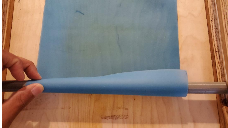
Figure 15: Wrapping silicon sheet around dowel rod
