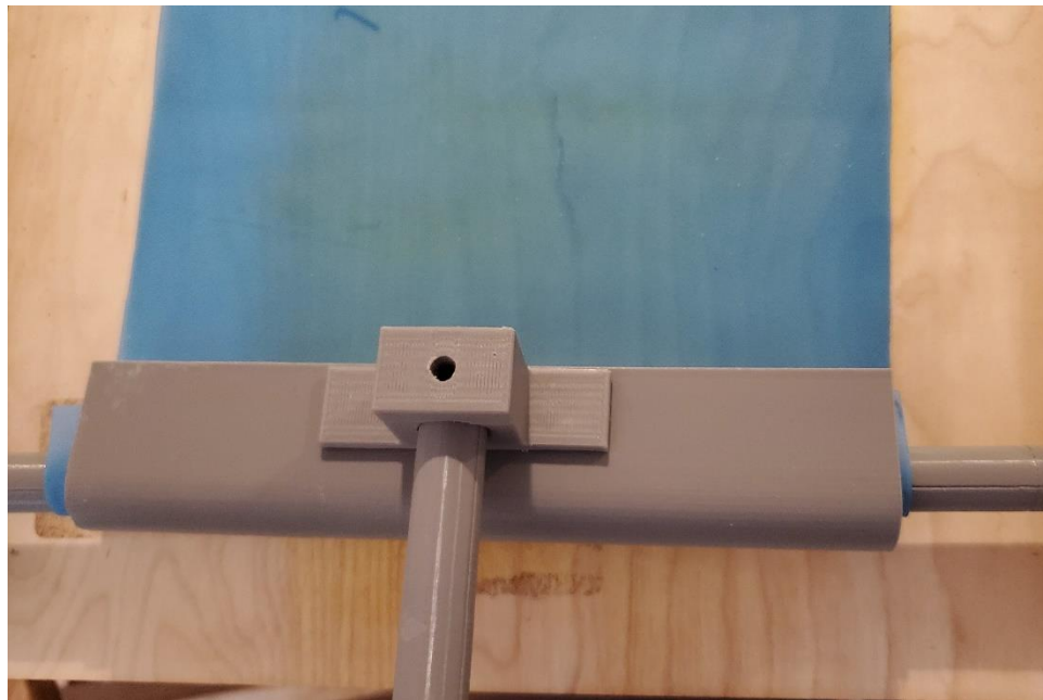
Figure 16: Pushing handle onto dowel rod
