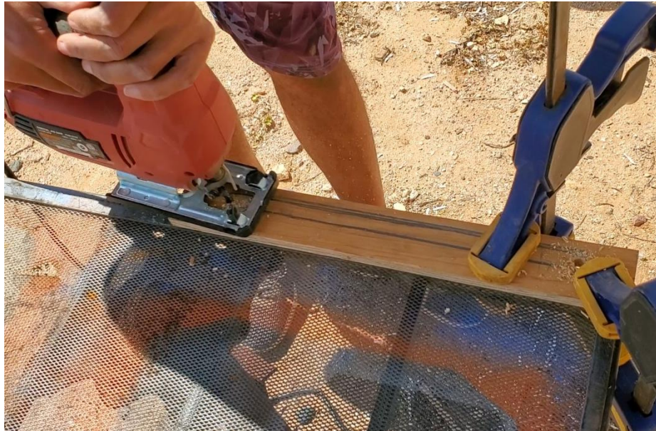
Figure 6: following the pencil line with a jig saw
