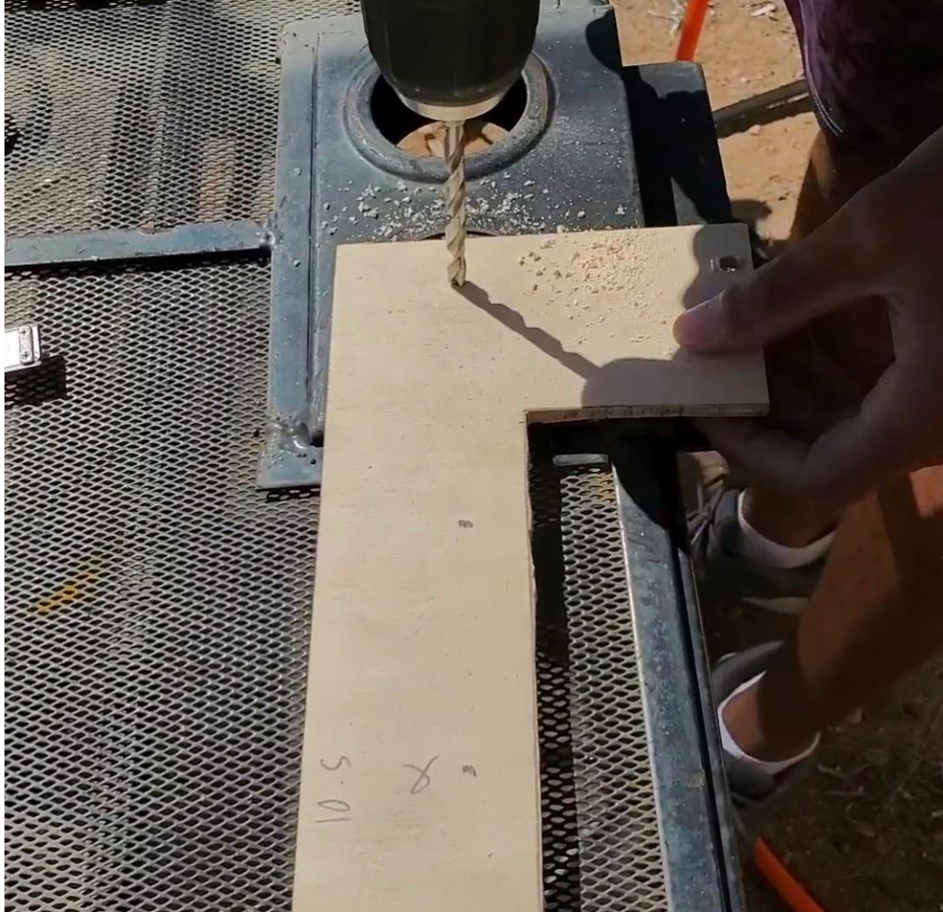
Figure 11: Drilling out holes in the end bracket
