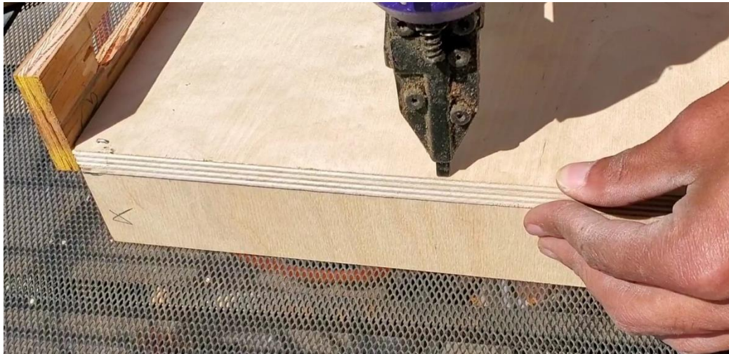
Figure 10: Placing the roller underneath the front edge and stapling them together
