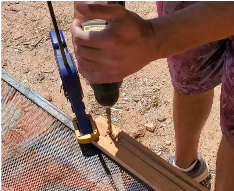
Figure 5: Drilling the two holes in a curved portion
