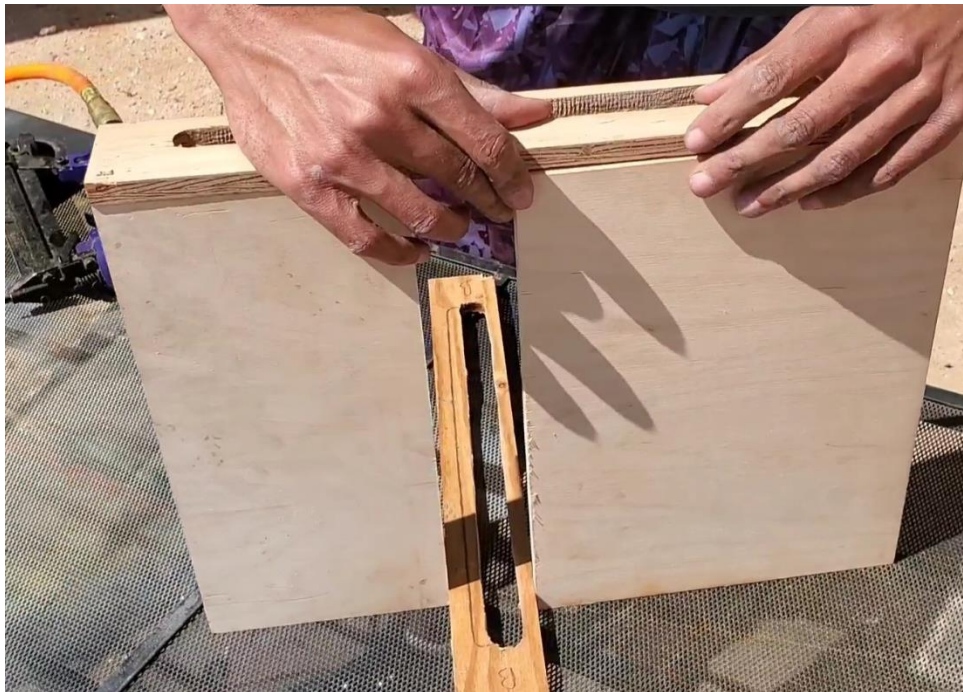
Figure 9: placing the other rail on bottom of the base and stapling it together
