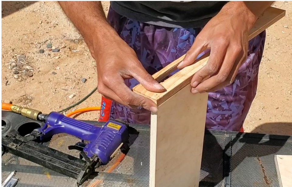
Figure 7: placing the rail on top of the base top
